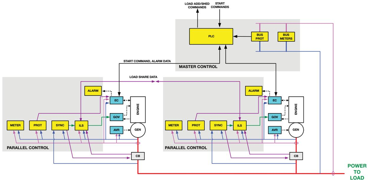
**Figure 3** - A block diagram of a simple isolated bus paralleling system showing interface of generator sets, paralleling functions and master control system. Note that the only interface between the generator sets is the load sharing signals.
