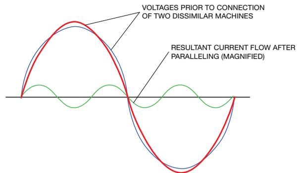
**Figure 1** - Whenever there is even an instant where the voltage between the two sources is different, current will flow between the machines.
